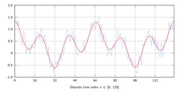
Signal y(n) reconstructed from cleaned spectrum
