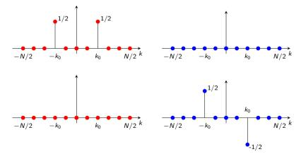
• Cosine is symmetric around k = 0. Sine is antisymmetric around k = 0.
