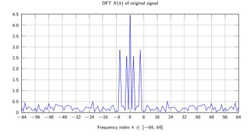
• How do we remove the noise?  $\Rightarrow$  Reshape the spectrum
