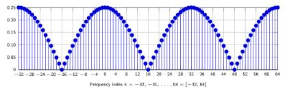
Modulus |X(k)| of the DFT of square pulse, duration N = 32, pulse length M = 2
